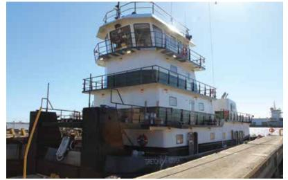
The vessel has the capacity of 44,200 gallons of fuel and 10,000 gallons of potable water, along with providing the maximum working draft. The MV GRETCHEN V. COOPER is outfitted with six crew staterooms housing eight crewman at a time, with four and a half baths and full galley arrangement.
